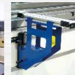
Adjustable Sliding Front Support Arms
