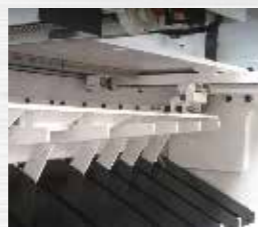
Pneumatic Sheet Support System
