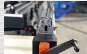
WILA TYP 'Opposing wave' Manual Crowning System
