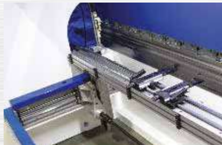
Heavy Duty Rigid Servo Driven 2 Axes X + R Back Gauge
