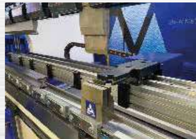
Heavy Duty Rigid Servo Driven 5 Axes X+X5+R+Z1+Z2 Back Gauge
